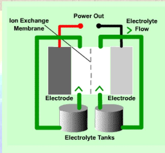
Modern flow cells are generally two electrolyte systems in which they act as liquid energy carriers, are pumped simultaneously through the two half-cells of the reaction cell separated by a membrane.
